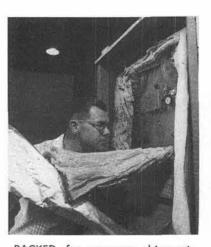
PACKED for overseas shipment, tape recorder is inspected by Arthur D. Bacon (3624-2). Wooden crate is painted with adhesive, lined with water-vaporproof paper. Next comes a lining of shock insulating material, then another foil-fabric-paper vapor barrier. Finally, the instrument itself, wrapped in a nest of crepe fiber.
